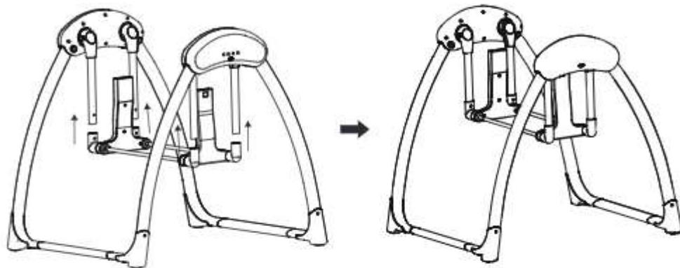
4. Unfold the cradle basket, open the zipper of the basket cloth cover, remove the inner fabric lining of the cradle basket, push the metal wires clip into the plastic holder on two sides. Then install the inner fabric lining and zip up the zipper. Unfold the canopy.
