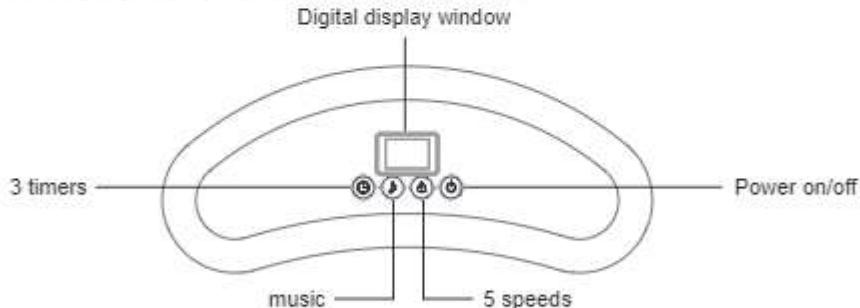
Power on/off: Press button, the cradle connects with power, and power light turns on.
