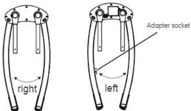
2. Assemble the bottom frame crossing tubes as shown in below figure, (pls attention right and left frame modules face inward as below figure ) Until the "click" sound indicates it is installed in place.
