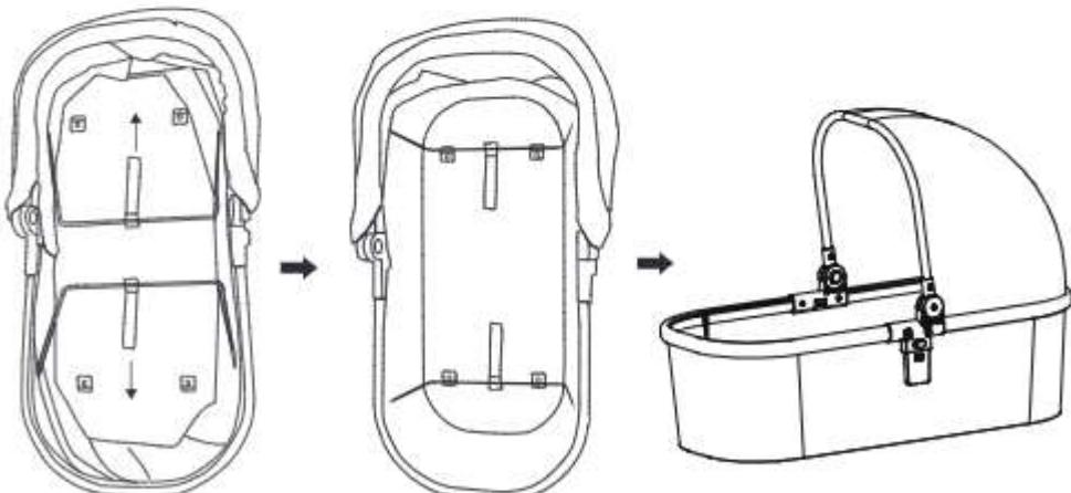
5.Put the cradle basket onto the frame. Align the two sides and insert into the plastic house on the cradle support base.Until "click" sound is heard, it means it is installed in place.
