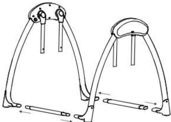
3. As shown in the figure, align the pipe orifices on the cradle module and insert them into the hanging tubes on the left and right frame module accordingly. Until "click" sound is heard, it means it is installed in place.
